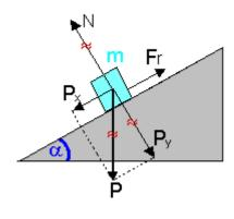
$$\begin{aligned} m \cdot a &= 5 \text{ kg} \cdot 0, 2 \text{ m/s}^2 = 1 \text{ N} \\ P_x &= P \cdot \cos \alpha = \text{ m} \cdot \text{g} \cdot \cos \alpha = 5 \text{ kg} \cdot 9,8 \text{ m/s}^2 \cdot \cos 37^0 = \\ &\qquad \qquad 39,13 \text{ N} \end{aligned}$$
